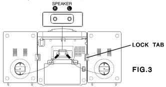
**NOTE:** This set can be used with speaker boxes attached to the main set or separated, just make sure both speaker plugs are plugged into the jacks.
